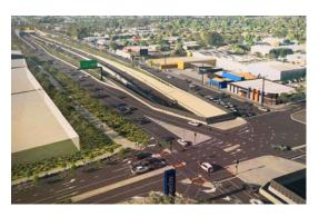
A technical review found that the tunnel portal needs to move approximately 300 metres to the north to improve traffic performance and safety. This design change will give motorists more distance and time to change lanes between Tonsley and the tunnel portal. It will provide better east-west connection via a shared-use bridge over the motorway, and reduce long-term closures of the Darlington motorway during construction.
